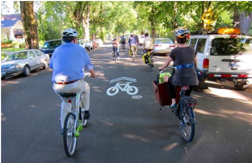
Figure 7. Bike boulevards include shared lanes on a low-volume, low speed street with bike and pedestrian prioritization features.
