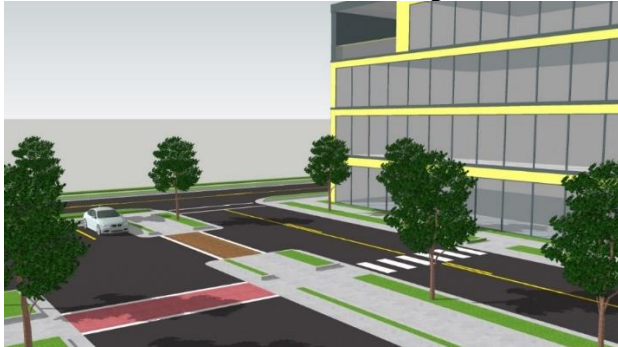
Figure 132. Allowed pedestrian crossing treatments are each represented in this figure. Pedestrian crossings include curb cuts and pathways through landscaped areas.
