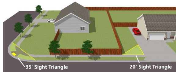
Figure 2. The 6-foot side yard fencing does not extend into the required 35-foot or 20-foot sight triangles. In this case, the 20-foot sight triangle does not interfere with the side yard fencing.
