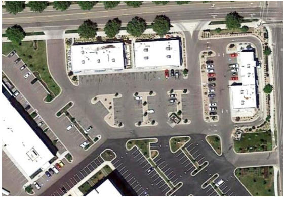
Figure 158. Adjacent nonresidential uses provide cross-access which reduces trips required on the surrounding streets.
