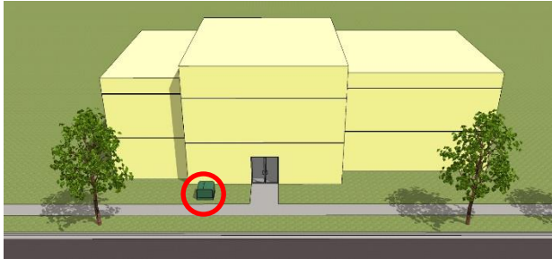
Figure 56 – Inappropriate example of a utility box being placed in front of the building.
