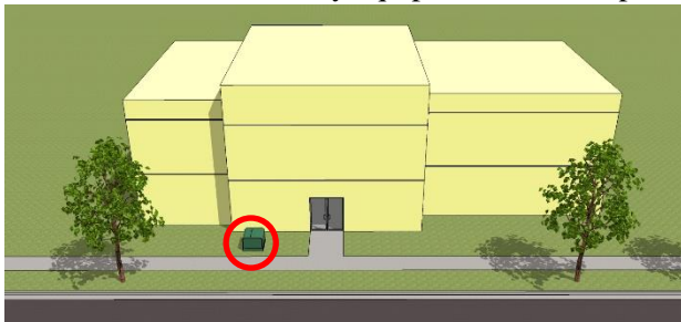
Figure 87 – Inappropriate example of a utility box being placed in front of the building.
