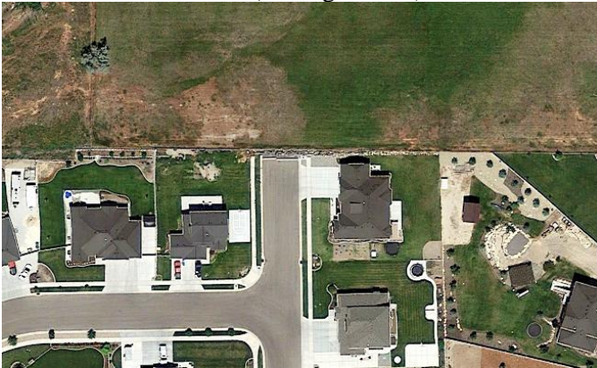
Figure 147. Example street stub intended to connect with a future subdivision on the adjacent undeveloped property.
