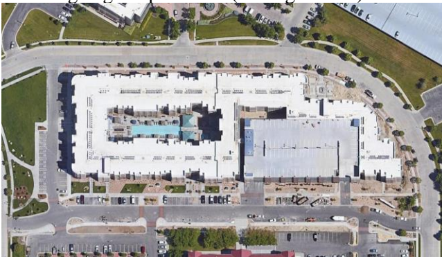
Figure 140. Apartment building has a common attached parking structure in lieu of individual unit garages.
