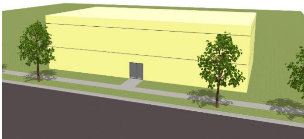
Figure 97 – Inappropriate example of a building with no articulations or roof line variations.
