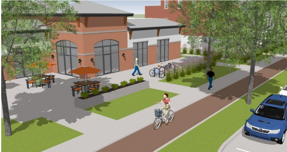
Figure 179. Bicycle parking is in a visible location near the building entrance in such a way it does not interfere with pedestrian traffic and has easy access to a protected bike lane.
