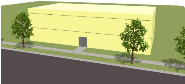
Figure 78 – Inappropriate example of a building with no articulations or roof line variations.
