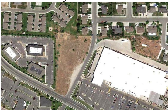
Figure 159. Local street stub connects a residential subdivision through a commercial site to an adjacent arterial street.
