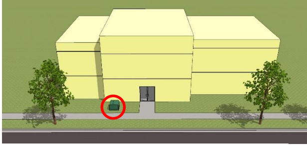
Figure 129 – Inappropriate example of a utility box being placed in front of the building.
